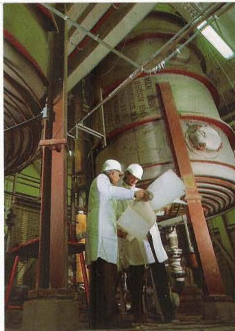
These semi-continuous edible oil deodorisers are part of a new oil processing department at Van den Bergh en Jurgens margarine factory at Nassaukade, Rotterdam, in the Netherlands. The equipment, which incorporates advanced automation, will give energy savings.
